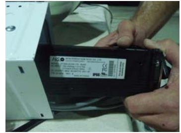
FIGURE 2: Inserting the drivers into the enclosure.
