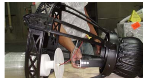
FIGURE 4: Installing the light bulb, diffuser, and driver.
