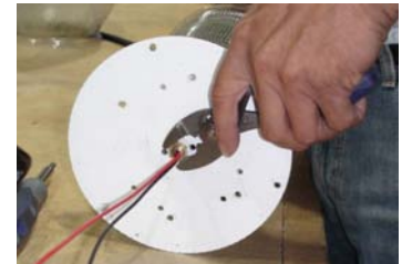
FIGURE 2: Securing the light bulb with a nut.
