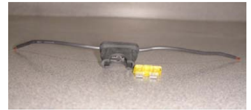
FIGURE 7: Wires on the left from the ULC that need to be connected to the solar panel.
