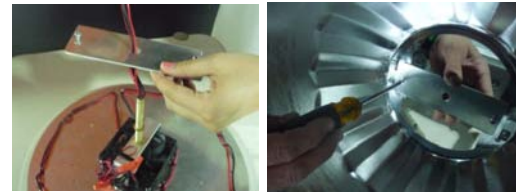
FIGURE 3&4: Removing the mounting plate from the bulb and attaching it to the reflector.
