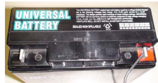
FIGURE 8: Connecting one end of the fuse holder to the battery.
