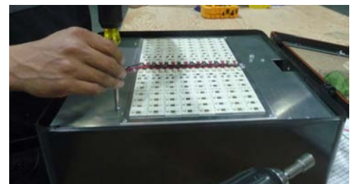
FIGURE 4: Inserting the bulb into the fixture.
