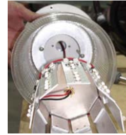
FIGURE 1: Inserting the light bulb into the diffuser.
