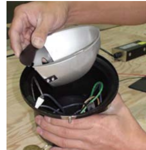
FIGURE 2: Removing the reflector from the housing.
