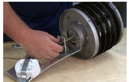
FIGURE 3: Installing light bulb into the diffuser.
