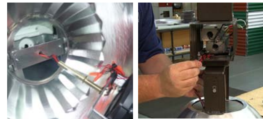
FIGURE 5&6: Inserting the bulb inside the reflector and routing the wires.
