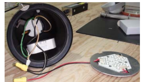
FIGURE 5: Wires connected from the bulb to the driver.
