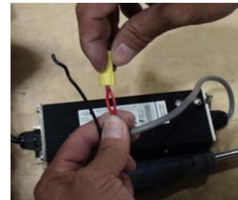
FIGURE 3: Connecting driver to light bulb.
